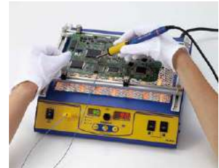
The temperature is regulated to match the preset value at the sensor location.
