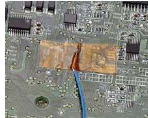
The sensor (thermocouple tip) is attached to the PWB.
